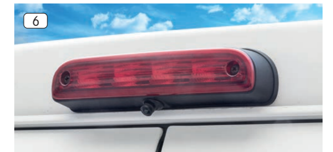
6. Align the cam housing / reflector assembly over the mounting location. Fix the assembly with the original Philips head screws.
