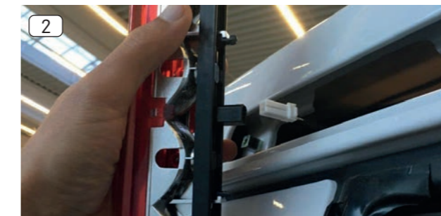
2. Pull the brake light reflector unit out of its mounting slot. Disconnect the white power supply system connector plug of the vehicle.
