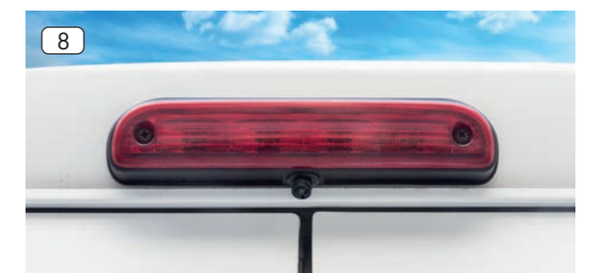
8. Perform a cam function test. Also check for proper function of the 3rd brake light. Align the camera sensor manually, for best desired image section. Installation and cam setup is completed.
