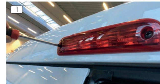
1. Unscrew and remove both Philips head screws. Retain the screws for later remounting of the brake light reflector.
